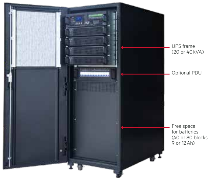
"Frame Plus" (UPS frame and batteries)
